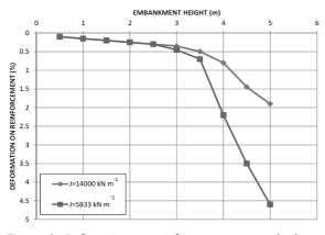
Figure 8. Deformation on reinforcement versus embankment height.
