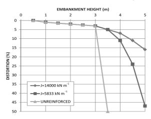
Figure 4. Distortion versus embankment height.
