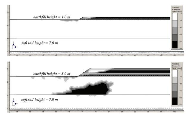
Figure 6. Geogrid with  $J = 14000 \text{ kN m}^{-1}$ .
