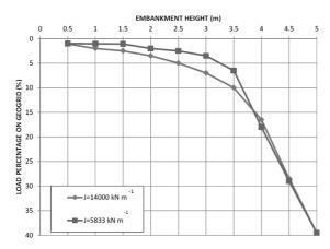
Figure 7. Geogrid load percentage versus embankment height.
