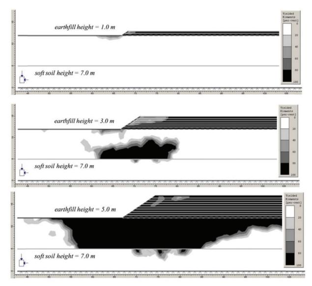
**Figure 5.** Geogrid with  $J = 5833 \text{ kN m}^{-1}$ .
