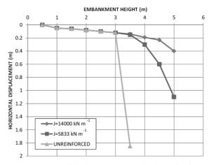
Figure 3. Horizontal displacement versus embankment height.
